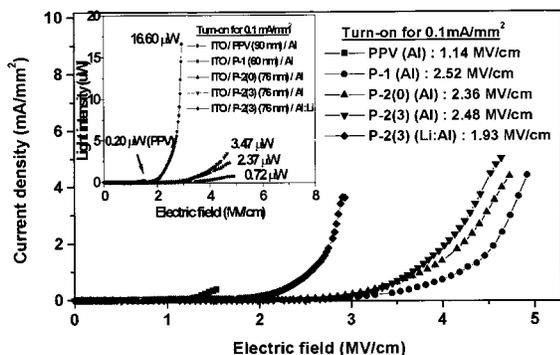
**Figure 6.** Comparison of  $I$ - $V$  and light intensity- $V$  curves for **P-1**, **P-2**, and PPV.
