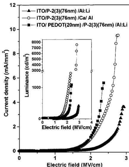
**Figure 8.** Comparison of  $I$ - $V$  curves and brightness of **P-2(3)** devices.
