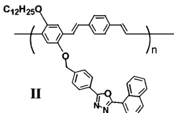
This polymer emits light at 580 nm, and the ITO/polymer/Al device exhibited an external quantum efficiency of 0.02% at a current density of about 8 mA/cm<sup>2</sup>. PPV itself shows the external quantum efficiency of about  $2.0 \times 10^{-4}$  to  $5.0 \times 10^{-4}$  % for the ITO/PPV/Al device.<sup>13</sup>
