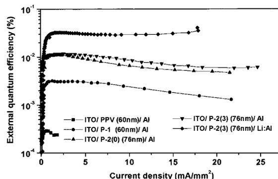
**Figure 7.** Comparison of current density-external quantum efficiency curves for **P-1**, **P-2**, and PPV.
